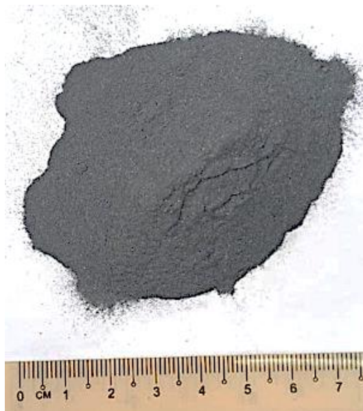
Figure 3: TiO 2 /ZnO feedstock powder for plasma spray process
