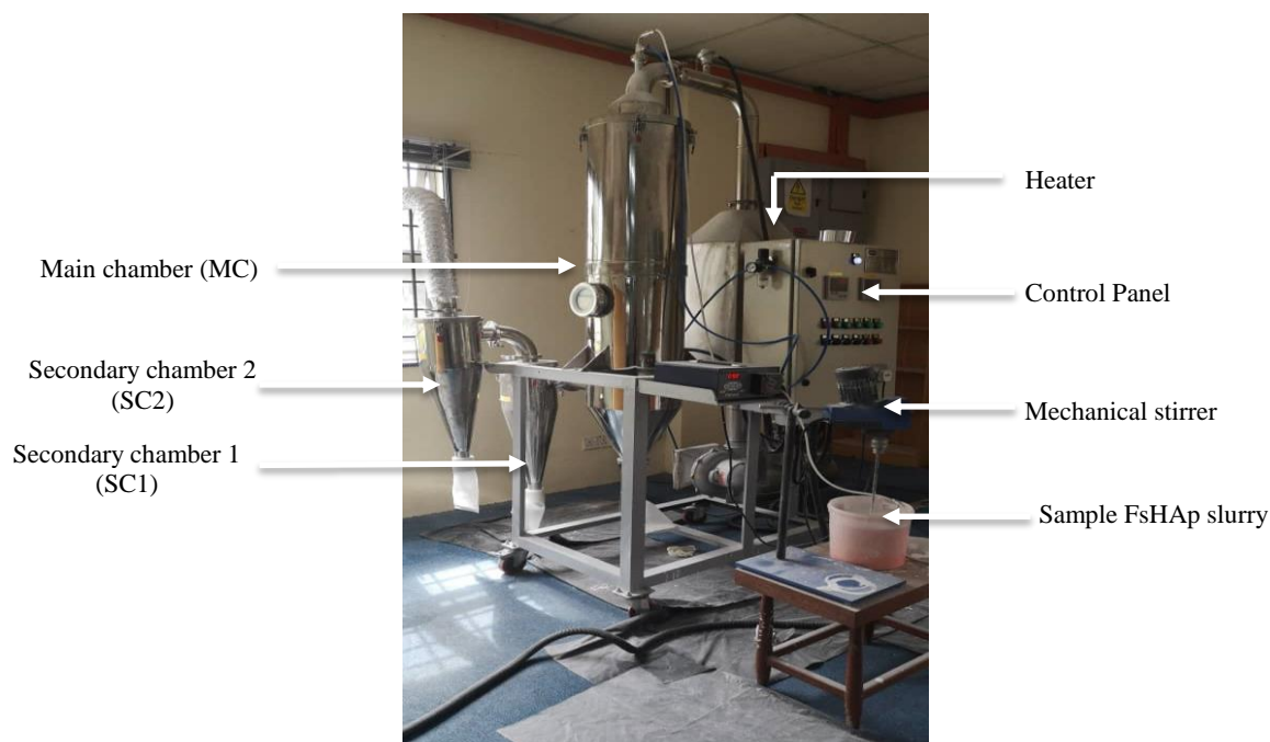
Figure 1. Spray dryer setup used in production of FsHAp powder
