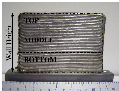
Figure 1 Photograph of the deposited Waspaloy plate showing (a) the top, middle and bottom sections transverse (T) to the build direction
