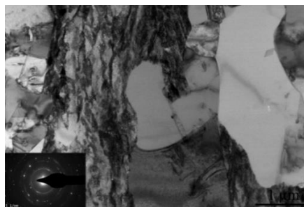
Figure 4: TEM image showing the microstructure of the Fe-17Mn-2Al-0.6C TWIP steel annealed at 575 °C
