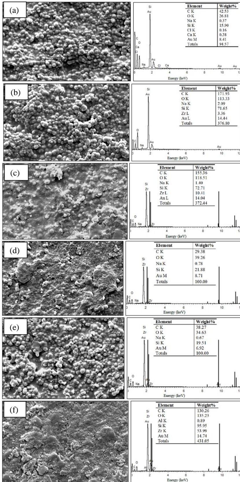
Figure 3 Representative of SEM micrographs on magnification of 20, 000x and EDS results: (a) CTX, (b) MM I 3% ZrO<sub>2</sub>, (c) MM I 5% ZrO<sub>2</sub>, (d) MM II 3% ZrO<sub>2</sub>, (e) MM II 5% ZrO<sub>2</sub>, (f) Z250 (3M, ESPE)
