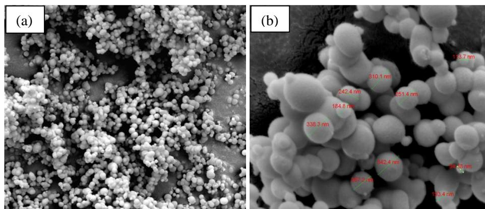
**Figure 2 SEM micrographs of nanosilica particle on magnification (a) 20, 000x and (b) 100, 000x**
