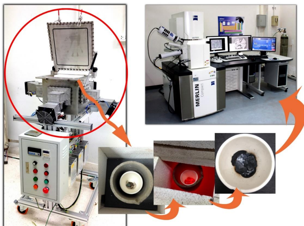
Figure 1. Alloying MnBi in microwave furnace and characterization by FESEM/EDS
