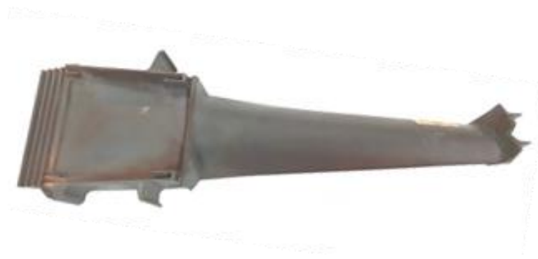
Figure 2. Used blade of GTD 111 EQX.
