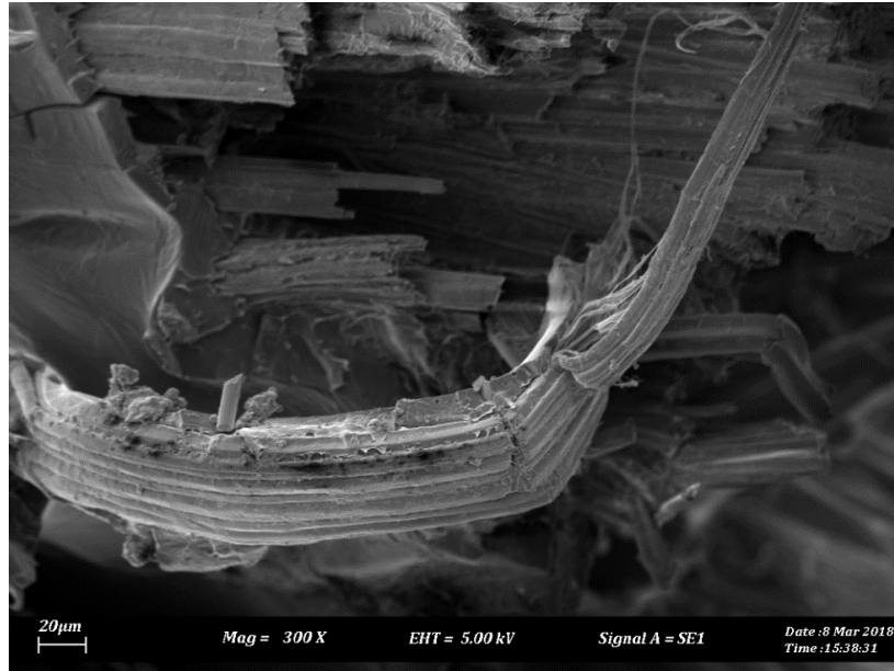
Figure 6. The presence of kink bank in 60 wt. % PALF/PLA composites
