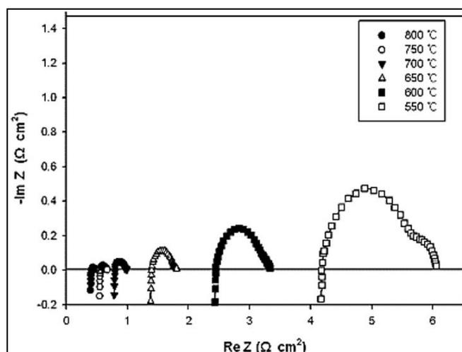
**Figure 13. The BSCZF05-SDC 30 wt% composite cathode impedance spectra plot at temperature 550 °C – 800 °C [50].**
