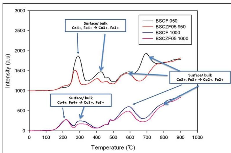
**Figure 9.** H<sub>2</sub>-TPR result curves for BSCF and BSCZF05 sintered at 950 and 1000 °C [50].
