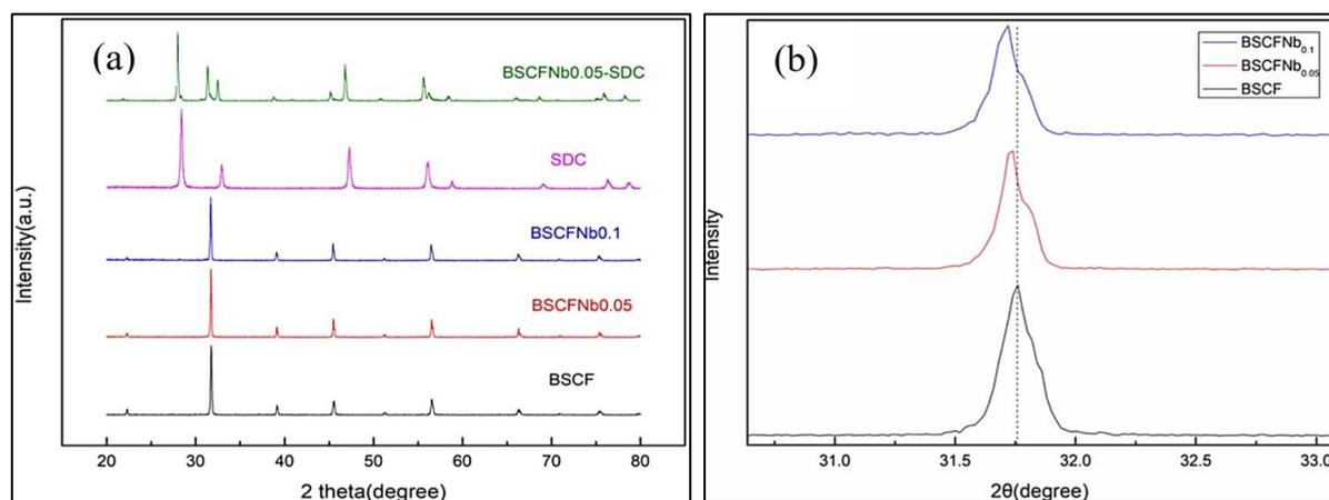
**Figure 1. (a) The XRD pattern of BSCF, BSCFNb0.05, BSCFNb0.1, SDC and BSCFNb0.05-SDC composite powder after 3 hours of calcination at 1000 °C and (b) Magnified image ( $2\theta = 31.7^\circ$ ) of XRD pattern for BSCF, BSCFNb0.05 and BSCFNb0.1 [38].**
