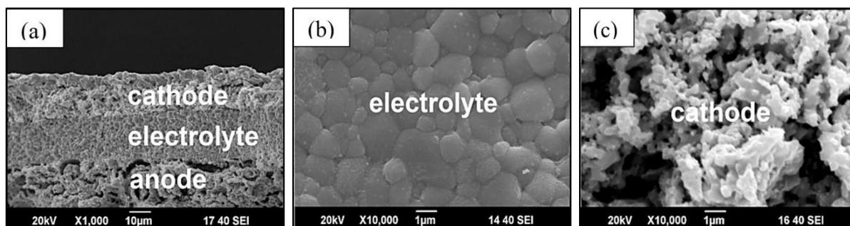
**Figure 2.** SEM image of (a) BSCFNb0.05 single cell structure in cross-sectional view, (b) SDS electrolyte surface morphology and (c) BSCFNb0.05 cathode in cross-sectional view [38].
