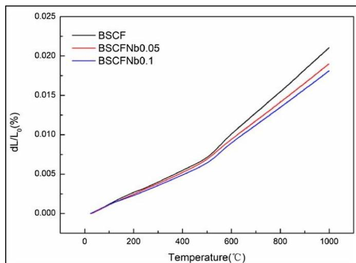
**Figure 4. The TEC curves of BSCFNbx samples with temperature measured in air Atmosphere [38].**
