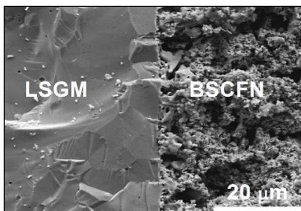
**Figure 3.** cross-sectional SEM morphology of BSCFN|LGS composite cathode [29].
