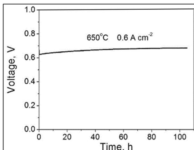
**Figure 6. The Ni-GDC|LDC|LSGM|BSCFN electrolyte supported cell voltage [23].**
