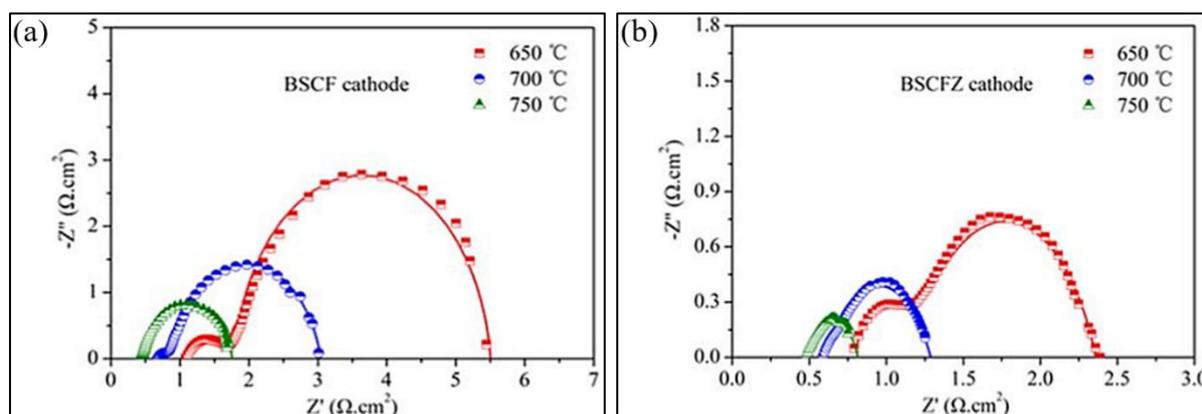
**Figure 11. Single cells impedance spectra results at operational temperature 650, 700 and 750 °C for (a) BSCF and (b) BSCFZ cathodes [34].**
