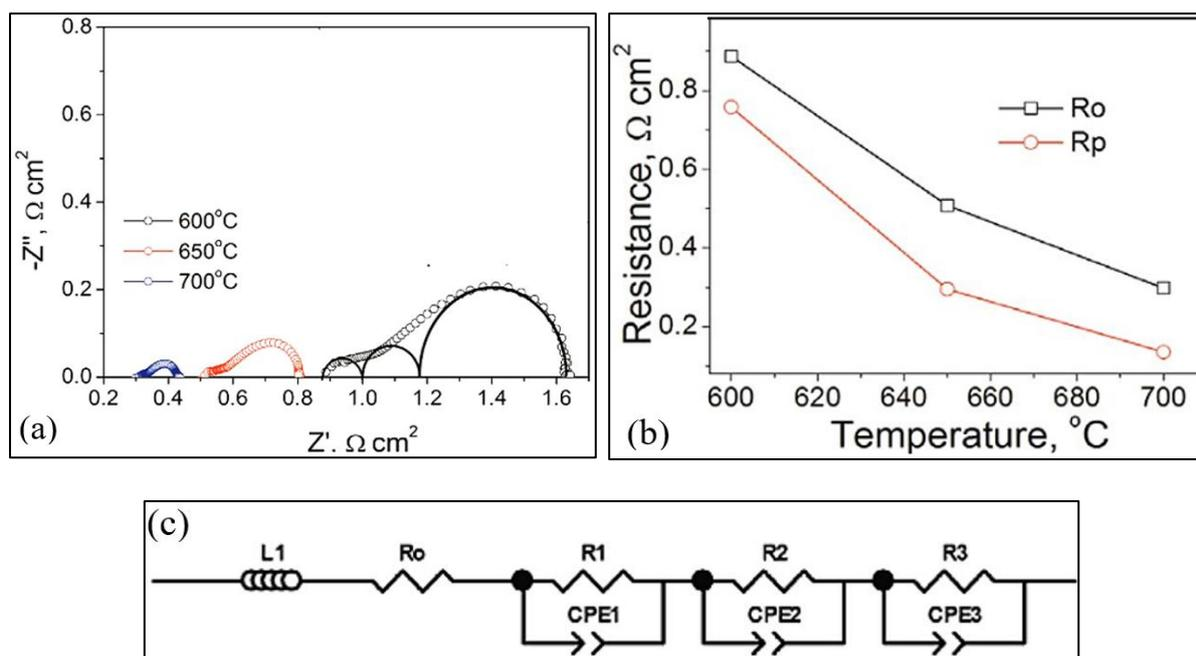
**Figure 5. The Ni-GDC|LDC|LSGM|BSCFN single-cell impedance spectra, (a) Fitted impedance spectra, (b) Illustration of  $R_o$  and  $R_p$  plots against operational temperature and (c) equivalent circuit [23].**
