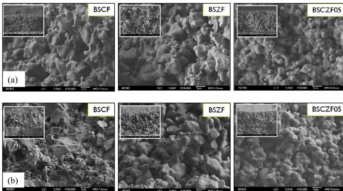
**Figure 8. SEM images of BSCF, BSZF and BSCZF05 cathode layer after sintering process at (a) 950 and (b) 1,000 °C [34].**
