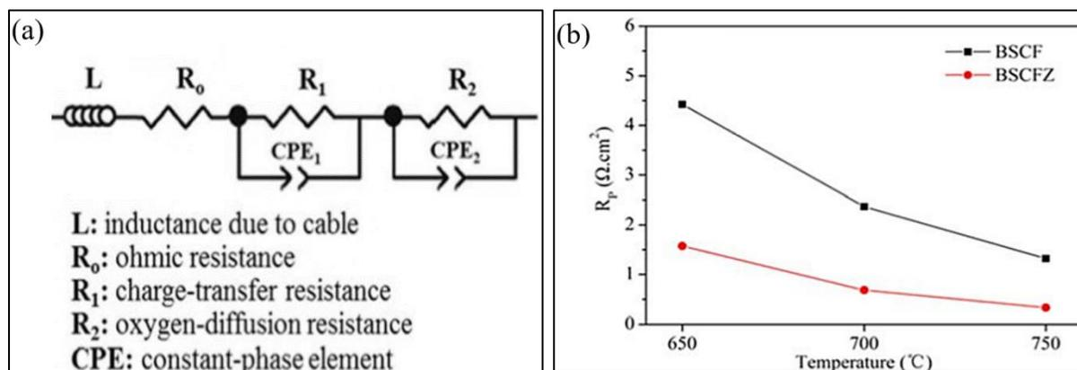
**Figure 10. (a) Equivalent circuit and (b) summarized Rp value for BSCF and BSCFZ [34].**
