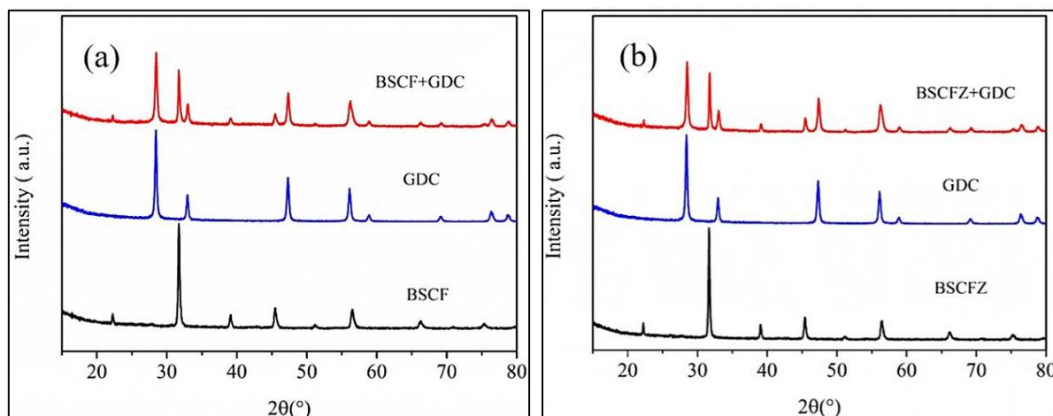
**Figure 7. The patterns of XRD for (a) BSCF, GDC and BSCF+GDC powder, (b) BSCFZ, GDC and BSCFZ+GDC composite powder fired in air for 6 hours at 1050 °C [34].**
