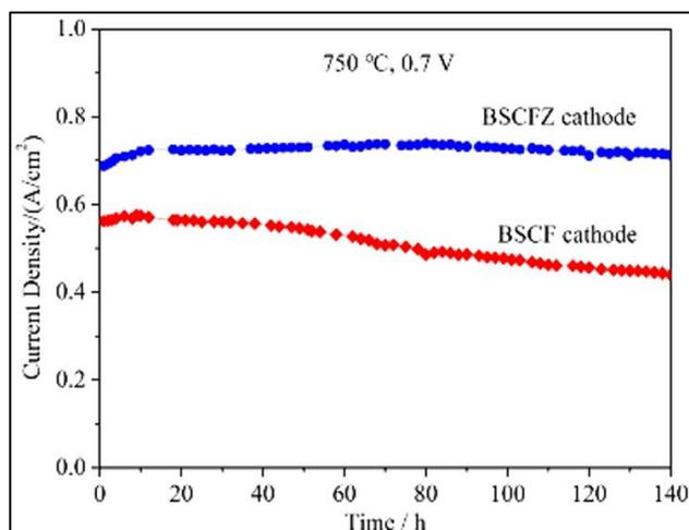
**Figure 12. Trend of current density for single cells with BSCF and BSCFZ cathode at 750 °C [34].**
