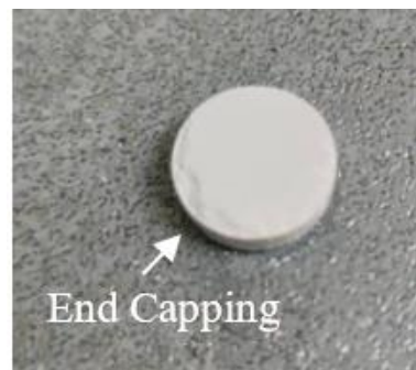
Figure 3: Observation of green compact pellet with end capping, uniaxially pressed under 250 MPa
