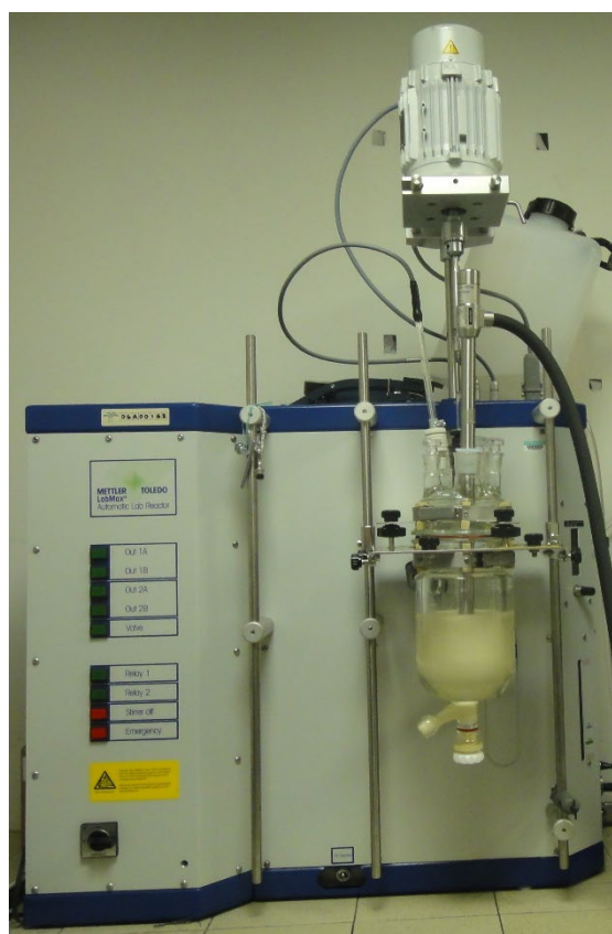
Figure 1: Fractional crystallization set-up with the FBRM probe
