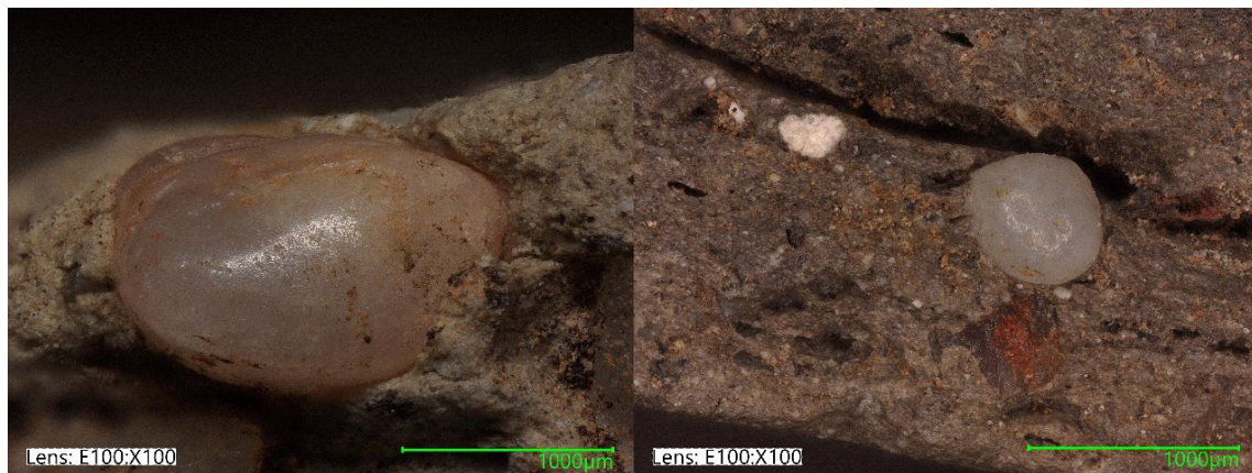
Figure 5(a): 2D images of quartz grain from the cross-section of sample GSa/Z5/S1/49 (right) and close-up view (left). The quartz grain is rounded in shape
