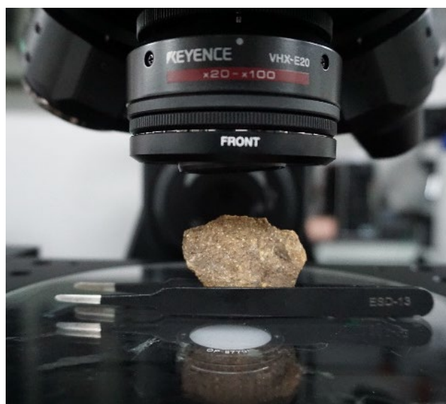
Figure 2: Sample setup position for cross-section analysis. The potshard was set up 90° on the stage in an upright position. The wide adjustable space between the stage and focal length of the microscope lens enabled accommodation of larger sample
