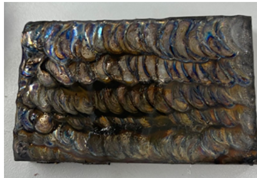
Figure 2: The composite coating sample on DSS with 50% overlapping weldment
