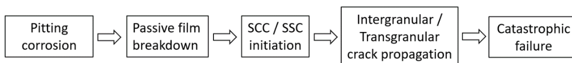
Figure 7: Schematic of the failure sequence in fuel tubes, progressing from pitting corrosion to SCC/SSC initiation, crack propagation, and final failure
